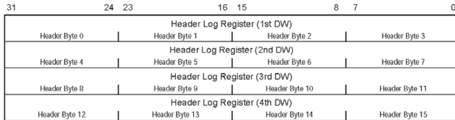
Figure 7-40: Header Log Register
